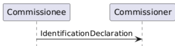
Figure 43. Overview of the UDC Protocol Identification Declaration message
